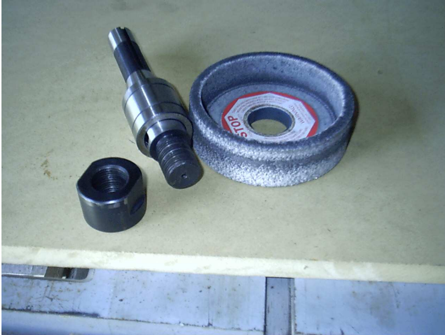
This is the R8 1 ¼ arbor and 5x 1 ½ x 1 ¼ white grinding wheel that will be needed to grind the broaches to size
